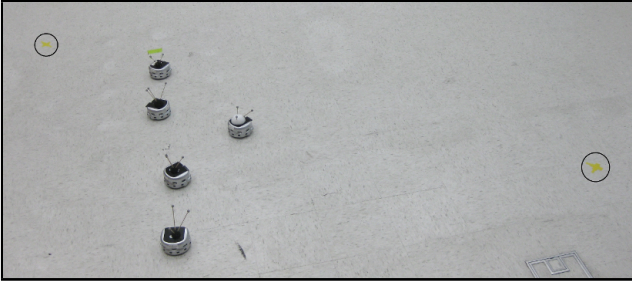
Fig. 3. Initial setup of the robot team, where the leader agent is the right-most robot. The two target locations are circled.
