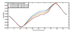
FIGURE 10. Forecasted original and PV embedded system profiles.
