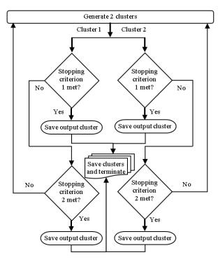
FIGURE 2. Extended k-means clustering algorithm flow chart [13].
