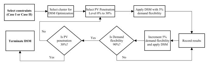
FIGURE 11. Selection of Cases (constraints) and, PV integration and demand flexibility level Scenarios for DSM applications.
