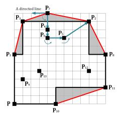
**FIGURE 11.** Path planning for multiple nodes classified to a same subpath.
