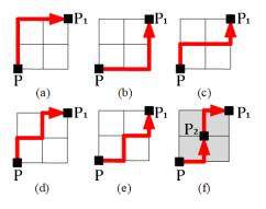
FIGURE 6. Several actual routes with the same shortest length between two nodes.
