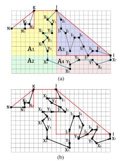
FIGURE 13. Path fusion process.
