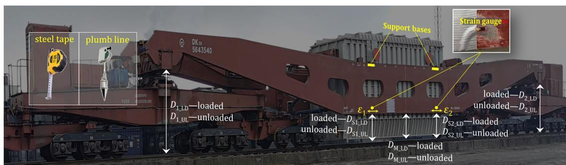
FIGURE 14. On-site measurement of static deflection and strains.
