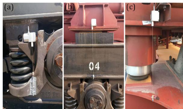
(a) Primary suspension, (b) second suspension, and (c) third suspension.
