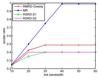
**FIGURE 6.** Percentage of admitted multicast destinations versus link bandwidth (40-nodes network with 20 multicast services and a per-service reliability requirement of 0.99).
