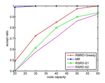
**FIGURE 9.** Percentage of admitted multicast destinations versus node capacity (40-nodes network with 20 multicast services and a per-service reliability requirement of 0.99, link bandwidth = 40).
