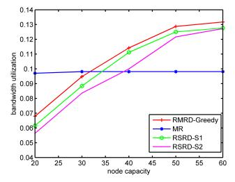
FIGURE 10. Bandwidth utilization versus node capacity (40-nodes network with 20 multicast services and a per-service reliability requirement of 0.99, link bandwidth = 40).
