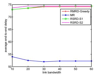
**FIGURE 8.** Average end-to-end delay versus link bandwidth (40-nodes network with 20 multicast services and a per-service reliability requirement of 0.99).
