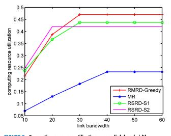
**FIGURE 7.** Computing resource utilization versus link bandwidth (40-nodes network with 20 multicast services and a per-service reliability requirement of 0.99).
