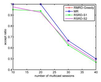
FIGURE 11. Percentage of admitted multicast destinations versus number of multicast sessions (40-nodes network with 10 - 40 multicast sessions and a per-service reliability requirement of 0.99, link bandwidth = 40, node capacity = 60).
