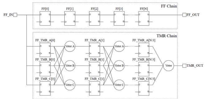
Fig. 8. Implemented Test Circuit: Standard Flip-Flop Chain and TMR Flip-Flop Chain
