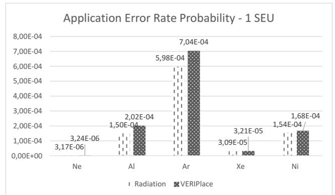
Fig. 10. A comparison of the Application Error Rate probability calculated from Radiation Experiments data and the VERI-Place tool.
