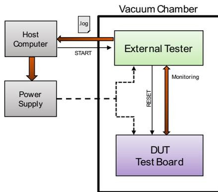
Fig. 7. Test setup with external tester in vacuum chamber.
