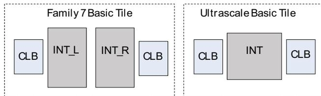
Fig. 1. Comparison between the Family 7 Basic Tile and UltraScale Basic Tile.
