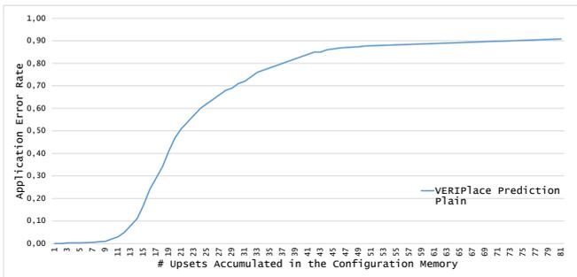
Fig. 9. Application Error Rate plot provided by the VERI-Place tool.
