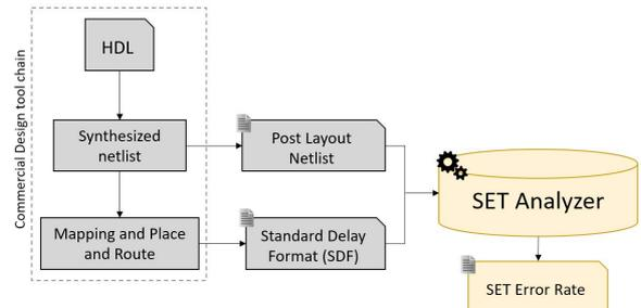
Fig. 4. Overall view of the developed flow for analyzing SET phenomena.
