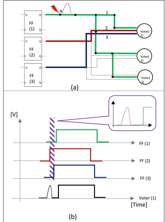
Fig. 3. Applied TMR methodology to a Single FF.
