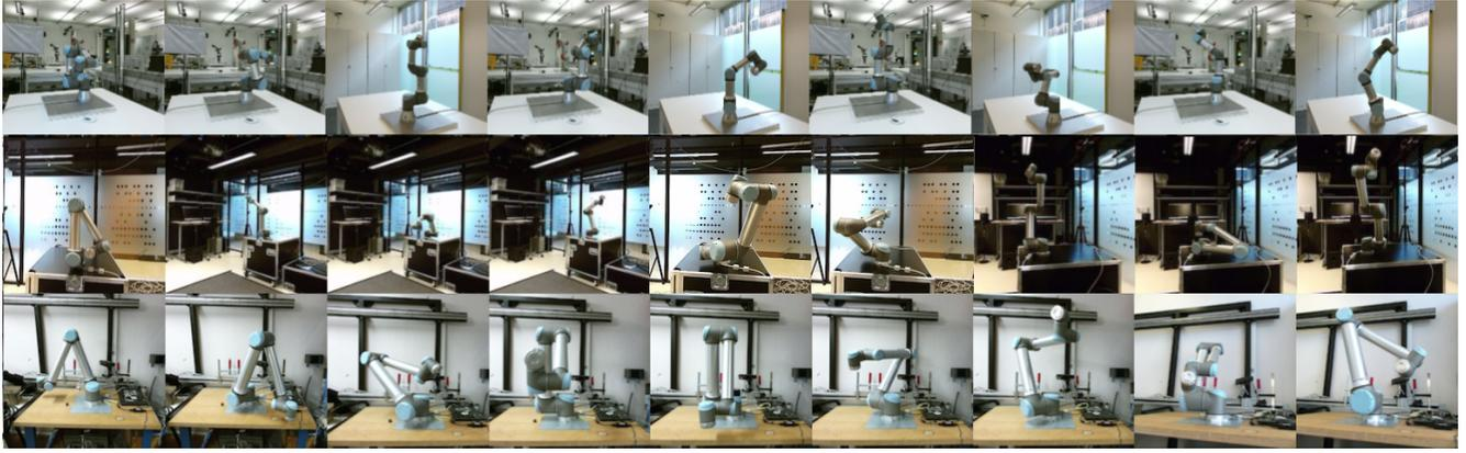
Fig. 1. Samples from a collected robot dataset. Each row of images represents different robot type in the following order: UR3, UR5 and UR10. The dataset was created using a varying background to provide more robustness.
