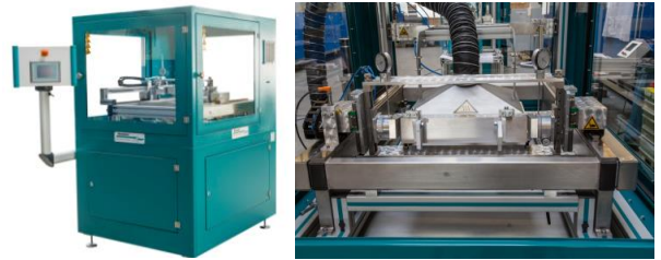
Figure 9. Discontinuous coating machine EC 63 for explosion protected printing of solvent-based inks and dispersions.
