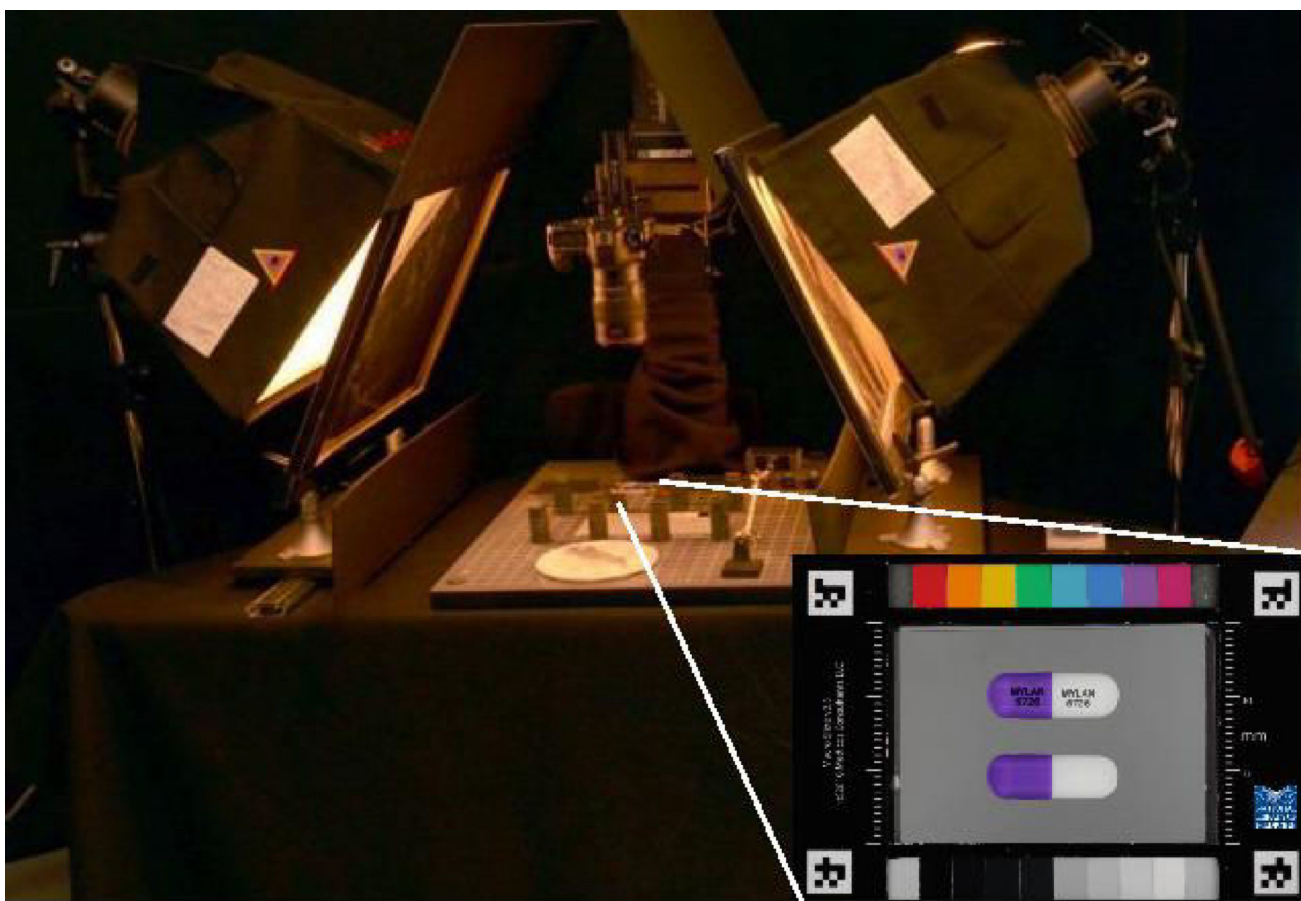
Fig. 1. Reference image macro photography rig. Inset shows the macro calibration card placed on top of floating stage and the imaged pills.
