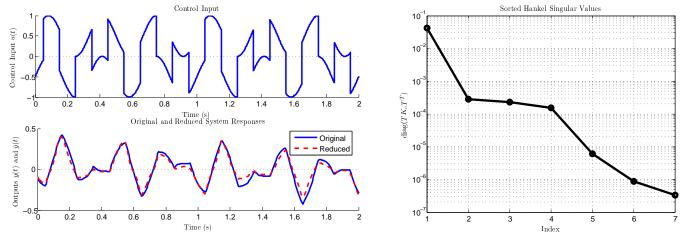
Fig. 1. (Left) Simulated output trajectories for the original and reduced (2-dimensional) system. (Right) Top Hankel singular values (zeros omitted).
