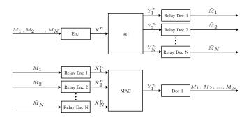
Fig. 2. The Chern–Özgür partial decode–forward coding scheme for L = 1.
