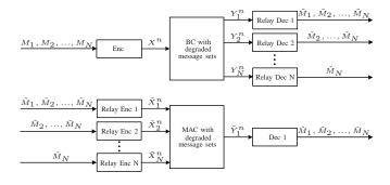
Fig. 3. The proposed partial decode–forward scheme for L = 1.
