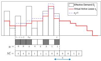
Fig. 2. An illustration of net incremental renting cost and wait time. When  $x_t < D_t$  ( $x_t \ge D_t$ ), i.e. the red graph is below (above) the black graph, a non-zero (zero) incremental renting cost is incurred. This is depicted using grey (white) epochs in the upper strip. In this example,  $\tau = 8$  and  $\eta = 3$ .
