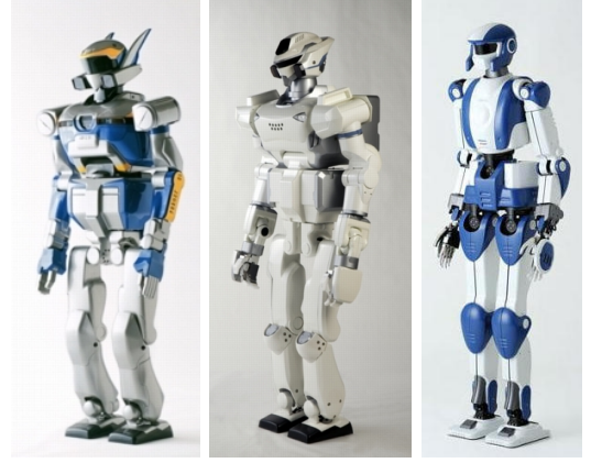
Fig. 1. Robots having similar kinematic structures but different velocity and joint limits
