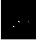
**First pass** Use high threshold to remove most irrelevant objects. Only objects with very similar colour of a typical ball left.
