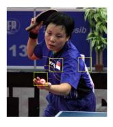
Second pass Use low threshold to enable the objects detected in first pass and their neighbourhoods to be fully revealed.
