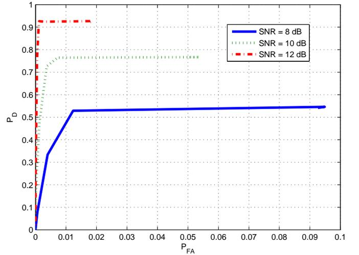
Fig. 4.  $P_D$  versus  $P_{FA}$  for different SNR.
