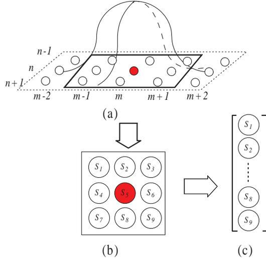
Fig. 2. An example of touch signal where the actual touch is on the sensor  $(m, n)$ : (a)  $3 \times 3$  sensors being affected by a touching finger with 2D Gaussian distribution of touch signal, (b) labeling the  $3 \times 3$  sensors in a vector form, and (c) rearranging the sensors in a vector form.
