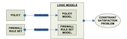
Figure 1. High level view of the firewall diagnosis process
