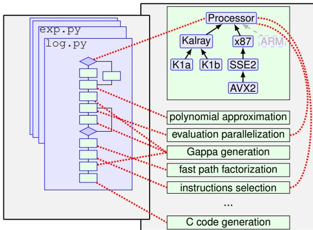
Figure 4: Zoom on the backend C code generator
