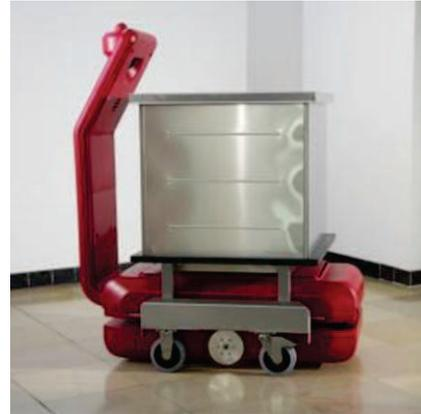
Fig. 1. Autonomous transport vehicle CASERO
