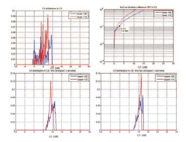
Fig. 3. Probability density function (PDF) of interference across the covered area (horizontal axis represents C/I, expressed in dB) in case: 1) all interferers are present (top-left), 2) the strongest interferer has been removed (bottom-left), 3) the two strongest interferers have been removed (bottom-right). The cumulative distribution function (CDF) of the difference between the two strongest interferers across the beam is also shown (top-right).
