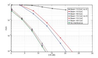
Fig. 9. Frame error rate for the reference signal using the simplified SIC scheme with one iteration (one detection and one decoding iteration). A 30 minutes LMS channel series in suburban environment generated according to [20] has been used. 10 interferers have been considered using the C/I values in Table II. Bearer F80T025Q1B-L8 (QPSK, channel code rate 1/3, symbol rate 8400 symbols per second) of standard [10] has been adopted for all signals.
