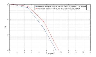
Fig. 6. FER in AWGN with MUD. Bearer F80T1Q4B-L8 (QPSK rate 1/3, symbol rate 33600 sym/sec, roll-off 0.25) is used for all signals. The interference pattern for beam 110 EoB detailed in Table II (worst case scenario) has been used.
