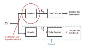
Fig. 4. Proposed SIC scheme. Only the strongest interferer is taken into account and no iterative detection is applied (i.e., reference signal is detected as described in Section III and decoded using the BGAN turbo decoder). Optionally also the strongest interfering signal can be decoded.
