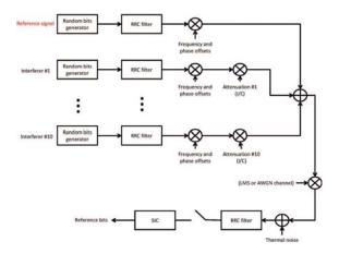
Fig. 5. Simulation setup in AWGN and LMS channels.
