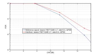
Fig. 7. FER in AWGN with MUD. Bearer F80T1Q4B-L7 (QPSK rate 2/5, symbol rate 33600 sym/sec, roll-off 0.25) is used for all signals. The interference pattern for beam 110 EoB detailed in Table II (worst case scenario) has been used.
