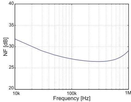
Fig. 3. The noise figure of SCF mixer.
