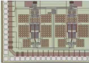
Fig. 4. Chip micrograph of SCF mixer.
