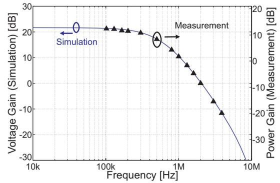
Fig. 5. Down-converted frequency response of implemented SCF mixer.
