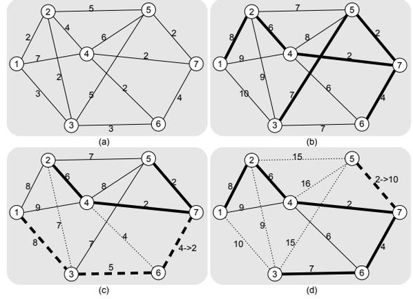
Fig. 5. A simple example of paths allocation with seven switches. (a) Initial network, the value on each edge  $e_{ij}$  is  $t_{ij}$ . (b) After  $InitSolve(7)$ , the value on each edge  $e_{ij}$  is  $dis_e(i, j, 7)$  and each bold edge  $e_{ij}$  means  $path(i, 7) = j$ . (c) Compare with (b),  $t_{67}$  decreases from 4 to 2, update some edges (labeled as dotted arrows). (d) Compare with (b),  $t_{57}$  increases from 2 to 10, update some edges (labeled as dotted arrows).
