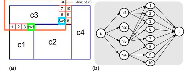
Fig. 4. A simple example of network interfaces insertion. (a)When  $l$  sets as the width of grid,  $l$ -box of core  $c3$  includes five free grids(label 1, 2, 3, 6, 7). (b) Corresponding network flow model.
