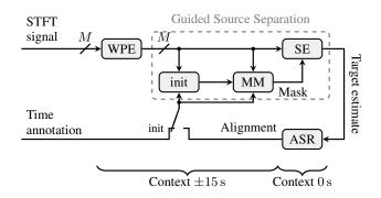
**Fig. 1**: Overview of speech enhancement system with Weighted Prediction Error (WPE) dereverberation, Mixture Model (MM) estimation, Source Extractor (SE) and Automatic Speech Recognition (ASR).
