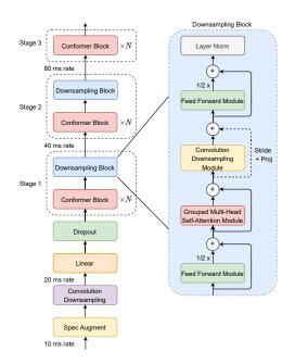
**Fig. 1. Efficient Conformer encoder model architecture.** The Efficient Conformer encoder is composed of three stages where each stage comprises a number of Conformer blocks using grouped attention. Encoded sequence is progressively downsampled and projected to wider feature dimensions.
