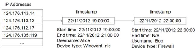
Figure 2. An example of the lookup table. The Source IP address 124.176.110.13 points to a list of sorted timestamp of labeled events; each points to the relevant username, end time and device type name.
