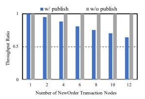
Figure 7: NewOrder transaction throughput ratio as a function of nodes, with and without publish.
