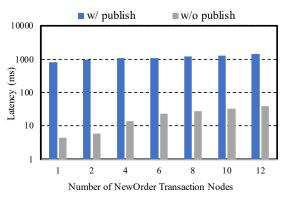
Figure 8: NewOrder transaction latency as a function of nodes, with and without publish.
