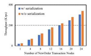
Figure 4: NewOrder transaction throughput as a function of nodes, with and without serialization.
