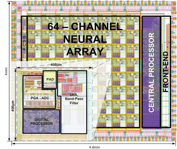
Figure 5. Layout of the multichannel neural sensor.
