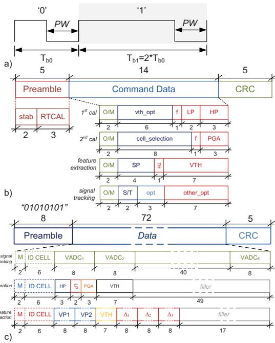
Figure 3. Communication protocol of the proposed system: a) PIE format, b) forward frame, c) backward frame.
