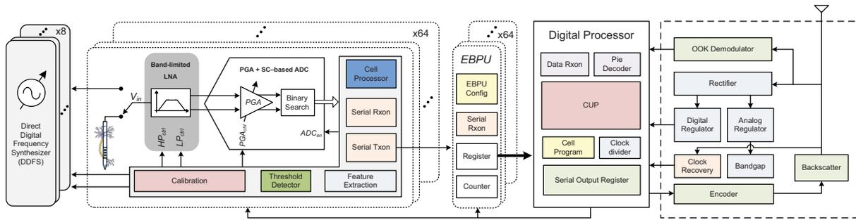
Figure 2. Architecture of the multichannel neural array.
