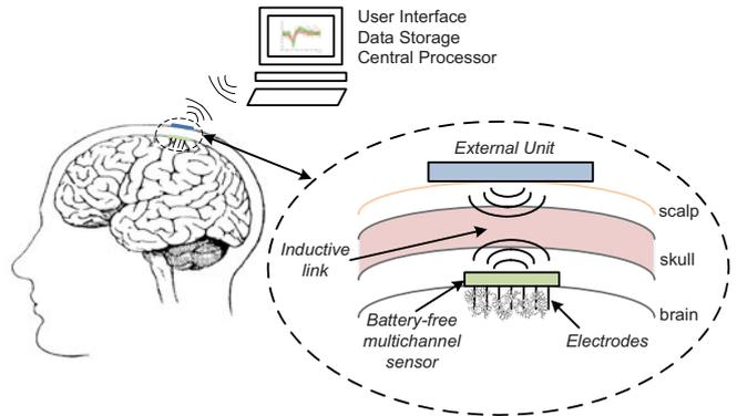
Figure 1. Implanted solution of the wireless neural array.
