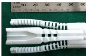
Figure 12: Laser sintered manipulator with two instrument arms and an additional arm in between with slots for two micro cameras.
