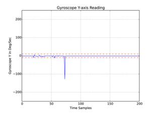
Figure 5. Gyroscope data (degrees/second) as a function of time measured during a dressing task showing when the sensor experiences motion outside of expected bounds (dashed lines).
