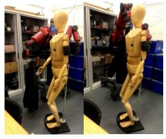
Figure 3. Sensor being tested during a dressing task. The sensor can be seen attached to the right arm near the end effector.
