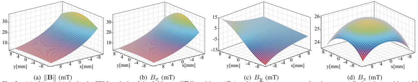
Fig. 3. (a), (b) and (c) depict the FEM analysis of the field norm ( $\|\mathbf{B}\|$ ) and its  $x$  ( $B_x$ ) and  $y$  ( $B_y$ ) components of an iron-core coil placed at position (-23 mm; 0 mm) with respect to the graph. The coil is controlled with a current of 1 A. Given the symmetry of the setup (Fig. 2), the field generated by the other coils can be obtained by properly rotating the ones shown here.
