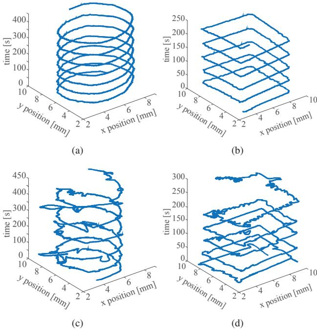
Fig. 4. Representative closed-loop motion control experimental results. Both trajectories are centered in (6 mm; 6 mm) with respect to the coordinates in the graph. In *a*) and *b*) the system operates in nominal conditions. In *c*) and *d*) an impulse-like disturbance is introduced every 3 s.
