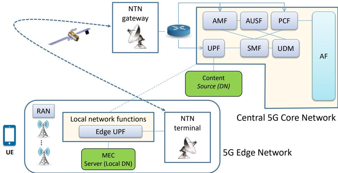
Fig. 1. Edge content delivery and offloading in 5G supported by satellite links
