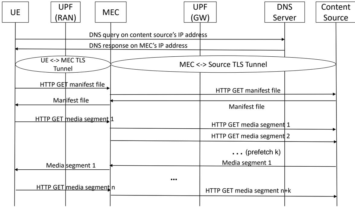
Fig. 2. Signaling sequence diagram for MEC prefetching
