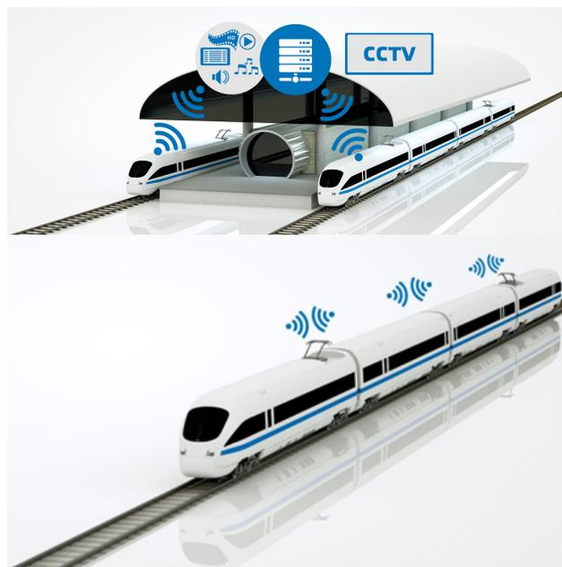
Fig. 1. Considered use cases of the high data rate link. Above: Transmissions from ground to train and vice versa. Below: Inter-carriage transmission.
