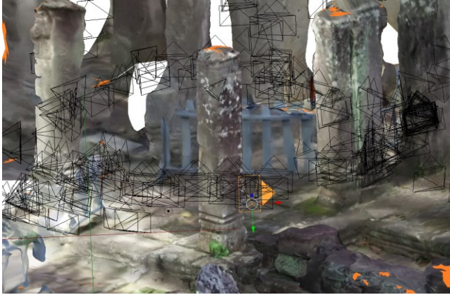
Figure 4. Virtual camera is installed at identical position as estimated camera position in generated 3D model space
