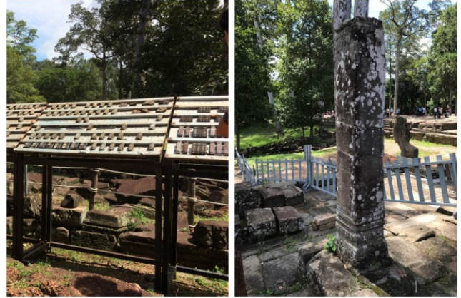
Figure 1. Different chemicals were applied to stones made of same material as ruins to observe progress. (Left: Various stone materials used for ruins, Right: Stone pillar of ruins of observation target)
