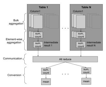
Fig. 4. Operation flow of mean aggregation
