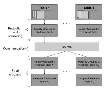
Fig. 5. Operation flow of Cylon group by operation
