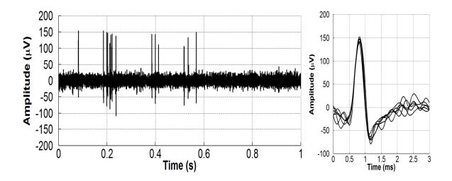
**Figure 2.9:** 1-second window of recorded data from the rat's cerebral cortex using the *SCI\_Gen1* and an expanded view of six neural spikes discriminated offline.
