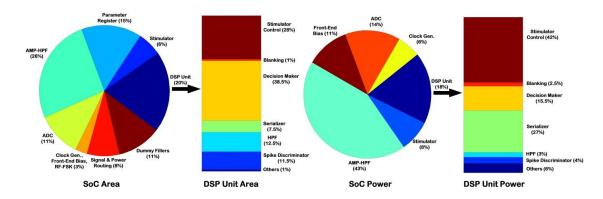
**Fig. 4.9:** Breakdown of silicon area (excluding I/O pads) and power consumption (excluding FSK-TX) for the BMSI and its DSP unit.
