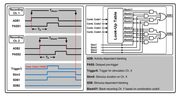
**Figure 3.41:** Individual blanking mechanism. SDB signals are generated from stim signals and combinations codes. Activation of ADB signals can blank the channels and also results in stimulation (activation of Stim signals). This again results in prolonged blanking by activating SDB signals in a blanking loop.
