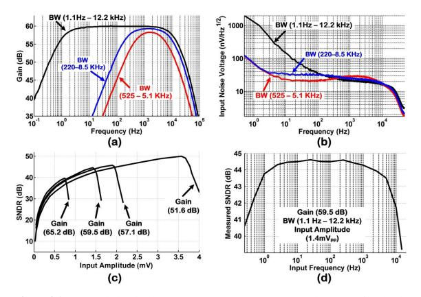
**Figure 4.6:** Front-end electrical measurements a) Frequency response b) Input referred noise voltage c) SNDR vs. input amplitude d) SNDR vs. input frequency.
