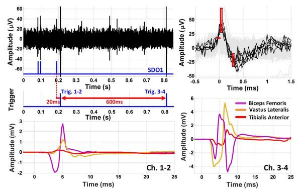
**Figure 4.11:** Closed-loop paired sequential ISMS; The BMSI was stimulating Ch.1,2 and Ch.3,4 with 600ms delay after successful discrimination of three neural spikes on recording Ch. 1.
