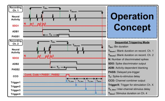
**Figure 3.1:** Conceptual illustration of the strategy for stimulus trigger generation from intracortical neural spike activity. A representative case involving two recording and four stimulating channels in sequential triggering mode is illustrated.
