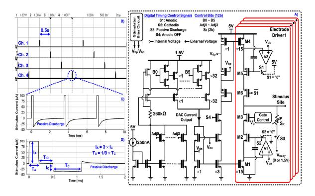
**Figure 2.3:** a) Circuit schematic of the stimulating back-end. b) Measured 4-channel sequential stimulation with a series resistive  $(1k\Omega)$ -capacitive (20nF) load. c) Measured train of 3 monophasic current pulses with passive discharge used in sequential stimulation. d) Measured asymmetric biphasic current pulse.
