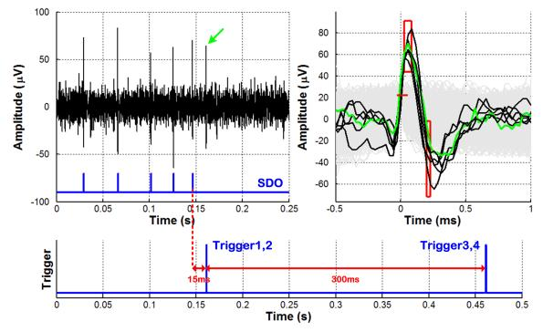
**Figure 3.9:** FPGA measurement results; Multichannel trigger generation for paired sequential triggering. Green spike occurred during the blanking period, so did not affect any ongoing process.
