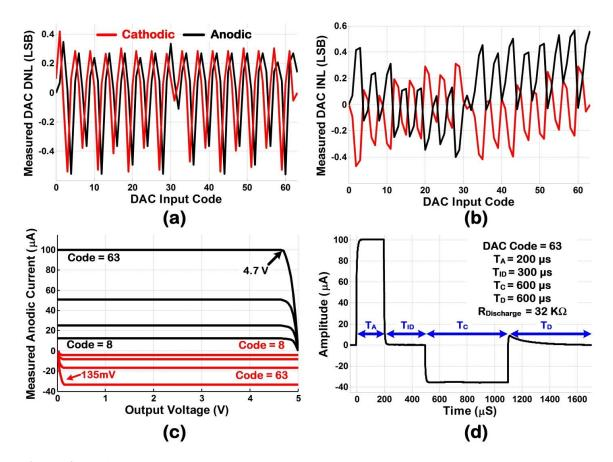
**Figure 4.7:** Stimulating back-end electrical characteristics; a) DAC DNL b) DAC INL c) output current versus output voltage for codes 63, 32, 16, and 8 d) asymmetric biphasic current pulse with the maximum amplitudes.
