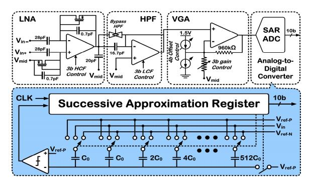
Figure 2.2: Circuit schematic of one channel in the recording front-end and the SAR ADC architecture.
