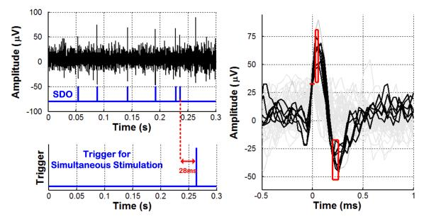
**Figure 3.10:** FPGA measurement results; multichannel trigger generation for simultaneous stimulation.
