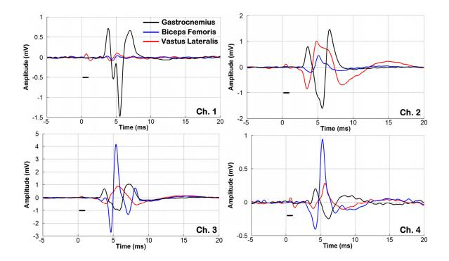
**Figure 2.81:** Recorded EMG signals from 3 hindlimb muscles activated via multichannel sequential ISMS in the rat's spinal cord using the *SCI\_Gen1*.
