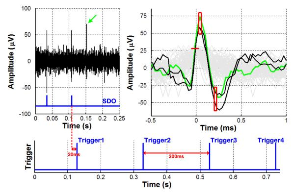
**Figure 3.8:** FPGA measurement results; Multichannel trigger generation for sequential stimulation based on discrimination of two intracortical neural spikes from a rat's cerebral cortex.
