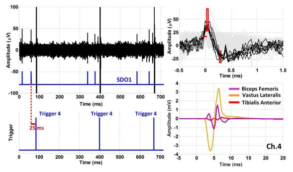
**Figure 4.10:** Closed-loop Individual ISMS on stimulating Ch.4 and resulted EMG signals; BMSI was stimulating Ch.4 after successful discrimination of two neural spikes on recording Ch.1.
