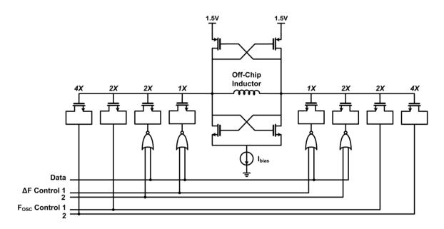
Figure 4.4: Circuit level schematic of the RF-FSK transmitter [4.3].
