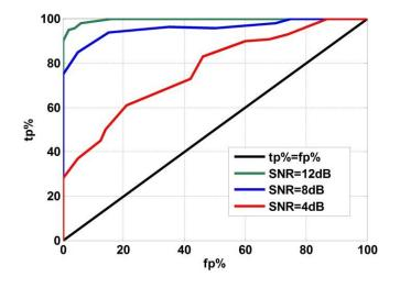
Figure 4.8: ROC curves for the implemented spike discriminator at three different levels of SNR.
