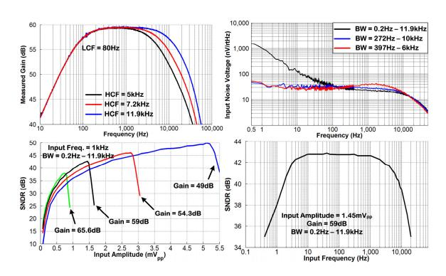
in 0.5Hz–50kHz was  $3\mu$ Vrms, leading to noise efficiency factor (NEF) of 2.47 for the LNA.
