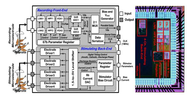
**Figure 2.1:** System architecture and die microphotograph of the *SCI\_Gen1* fabricated in 0.35µm AMS 2P/4M CMOS technology.
