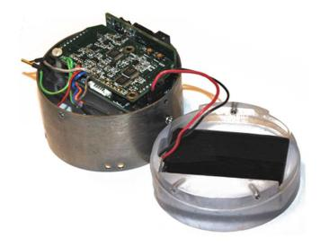
Figure 1.2: Neurochip-II device inside the titanium casing [1.29].
