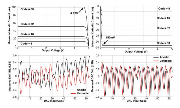
**Figure 2.6:** Top – Measured stimulator output current vs. output voltage in anodic (left) and cathodic (right) phases. Bottom – Measured DAC INL (left) and DNL (right) in both anodic and cathodic phases.
