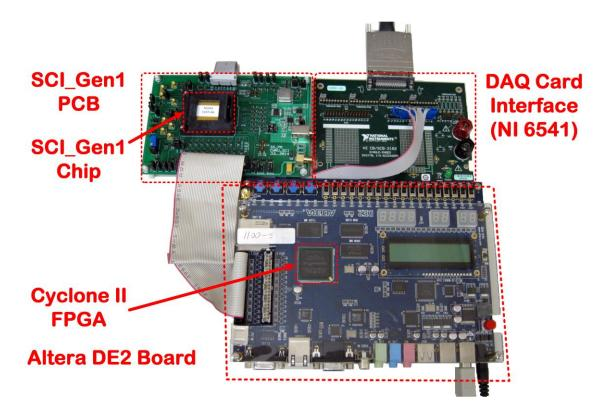
**Figure 3.7:** The measurement setup; prerecorded data is amplified by the chip and serves as the input for implemented algorithm on FPGA. Generated triggers are fed back to the chip for delivering charge balanced biphasic or monophasic stimulation pulses with passive discharges.
