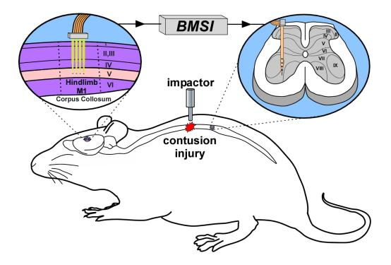
**Figure 1.3:** Conceptual illustration of our proposed brain-machine-spinal cord interface (BMSI); closed-loop intracortical control of intraspinal microstimulation (ISMS)
