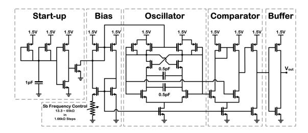
Figure 4.3: Circuit schematic of the clock generator with nominal frequency at 1 MHz [4.3].
