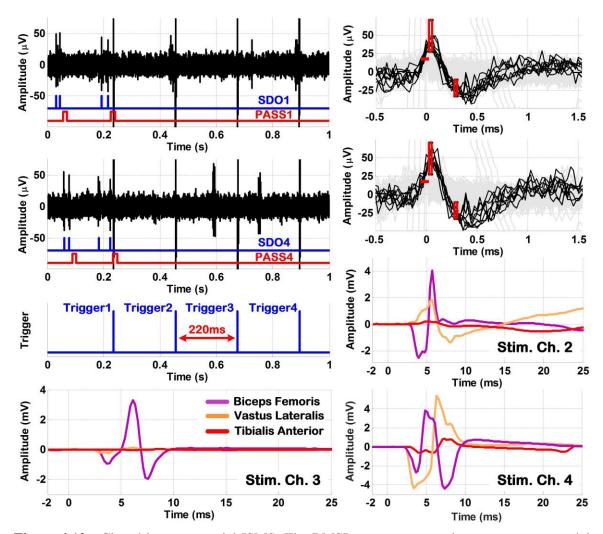
**Figure 4.12:** Closed-loop sequential ISMS; The BMSI was programmed to generate sequential ISMS when trigger-generation criteria were simultaneously satisfied on both Ch.1 and Ch. 4 (within a 15ms window), with sequential triggering criteria defined as the logic AND function of PASS1 and PASS4 signals.
