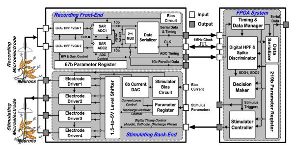
**Figure 3.6:** System architecture of the interfaced *SCI\_Gen1* device and reconfigurable FPGA platform for real-time ISMS trigger generation.
