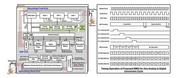
**Figure 4.1:** Proposed system architecture and timing diagrams of the proposed *SCI\_Gen2* BMSI system. There are two identical four-channel modules in the BMSI that share a clock generator, biasing circuit, and a FSK-TX.
