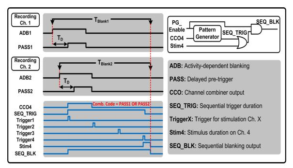
**Figure 3.5:** Sequential blanking mechanism illustration. Activation of ADB signals can blank the channels and also might result in sequential stimulation which ultimately leads to blanking all the channels for the entire stimulation period. Blanking starts at different time but ends simultaneously for all the recording channels.
