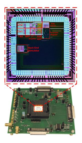
**Figure 2.4:** Top – Photograph of the custom PCB developed for biological tests and a die microphotograph of the  $2.9 \times 2.9 \text{ mm}^2$  SoC fabricated in AMS  $0.35 \mu m 2P/4M$  CMOS.
