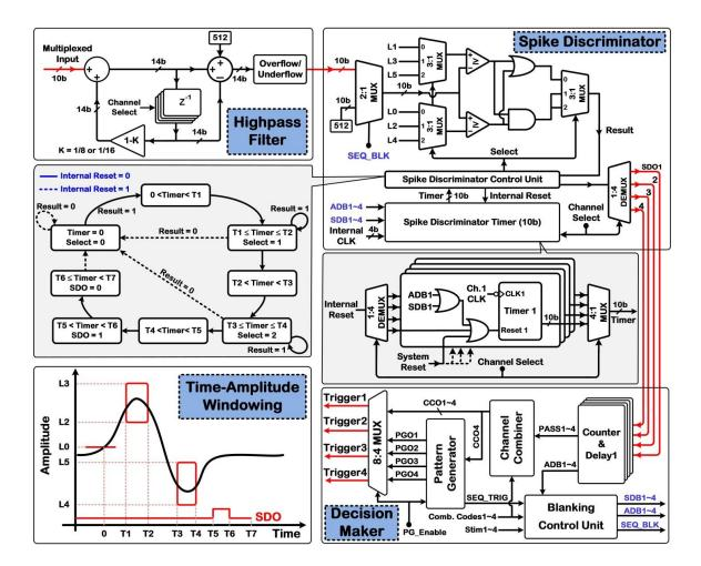
**Figure 4.2:** Detailed architecture of HPF, spike discriminator, and decision maker of the proposed DSP unit of the BMSI system along with finite state machine (FSM) representation of the spike discriminator control unit and timer structures.
