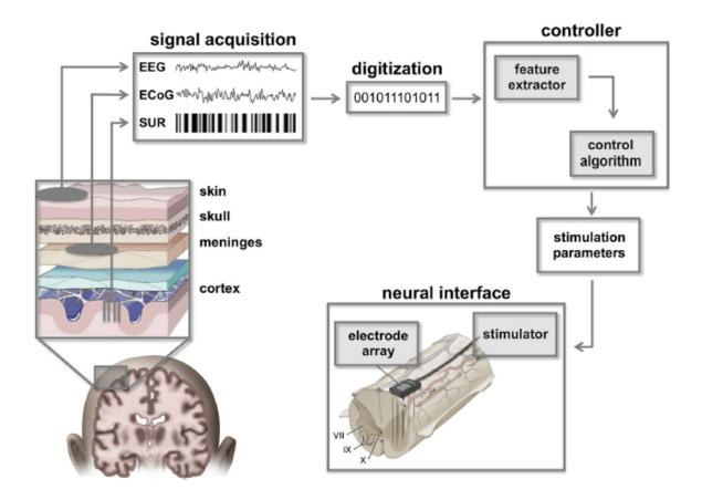
Figure 1.1: Conceptual illustration of a brain-machine-body interface (BMBI) [1.9]
