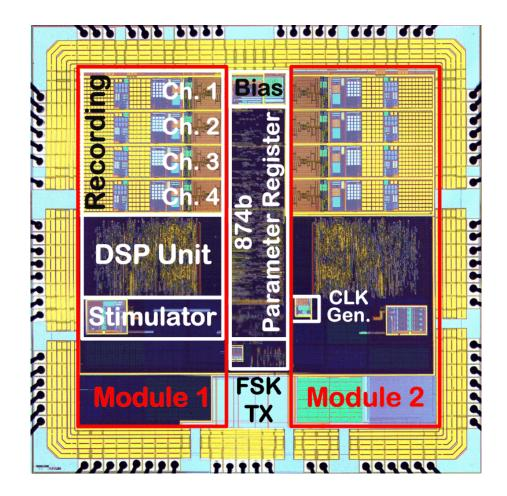
Figure 4.5: Die microphotograph of the SCI\_Gen2 BMSI in 2P/4M AMS 0.35um CMOS.
