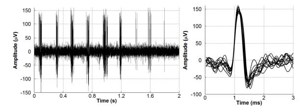
**Figure 2.7:** 2-second window of recorded data from the rat's cerebral cortex using the *SCI\_Gen1* and an expanded view of 12 neural spikes discriminated offline.
