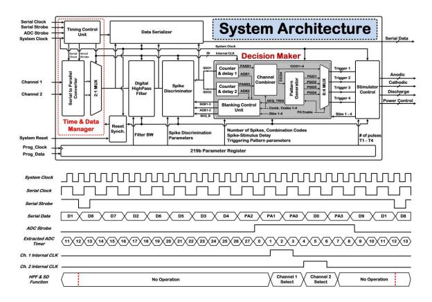
**Figure 3.2:** System architecture and timing diagram for hardware realization of the strategy for stimulus trigger generation from intracortical neural spike activity.
