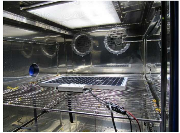
Figure 1. Solar panel in the climatic chamber for characterization
