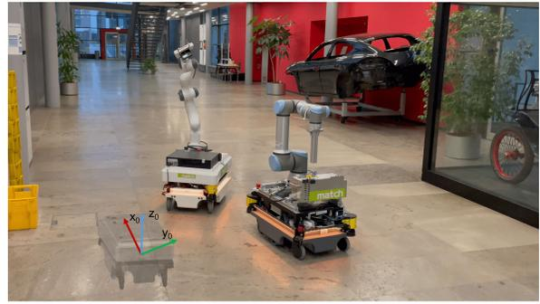
Fig. 7. Triangular formation of three MiR industrial robots. The three robots from left to right are: virtual leader, robot 1, robot 2
