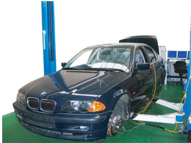
Figure 6.1: Front view of prototype brake-by-wire vehicle in HiL simulation set-up
