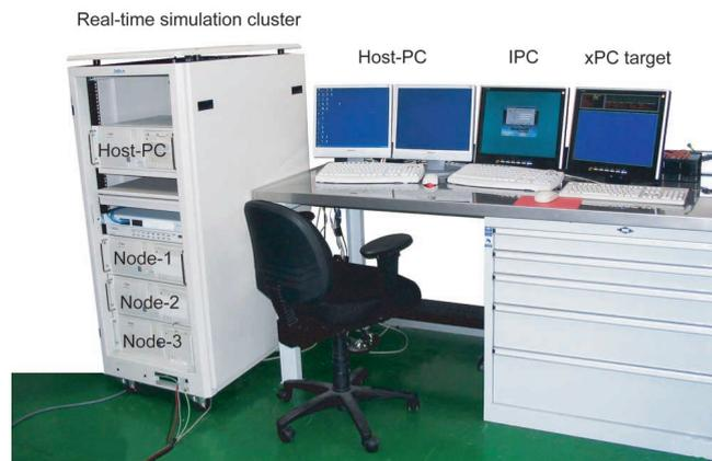
Figure 6.3: Picture of real-time simulation cluster with test bench
