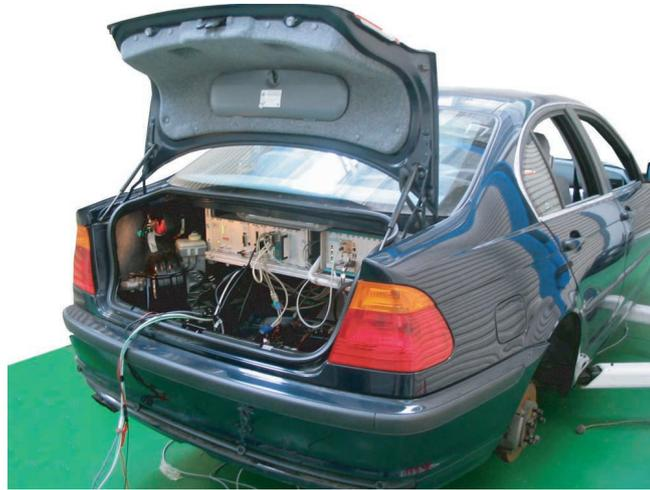
Figure 6.2: Rear view of prototype brake-by-wire vehicle in HiL simulation set-up
