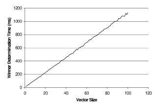
Figure 3. The effect of increasing weight collection size on winner determination time
