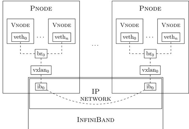
Figure 1. Network stack of a virtual node when using VXLAN encapsulation. Each virtual node has a virtual interface ( $veth_i$ ) that is bridged with VXLAN interface ( $vxlan_0$ ) on each *pnode*. This interface is associated with physical IP interface ( $ib_0$ ). In our study IPoIB is used, but more traditional IP over Ethernet can be used as well.
