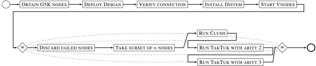
Figure 2. Experimental workflow. After the infrastructure is prepared (the first line of the workflow), a varying number of nodes ( $n$ ) is used to run Clush and TakTuk methods in a simple loop (denoted with “=”). At each iteration, the Distem infrastructure is analyzed and failed nodes are discarded if necessary.
