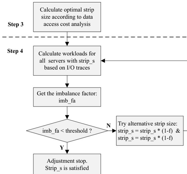
Fig. 4. Balance I/O workload by adjusting stripe size
