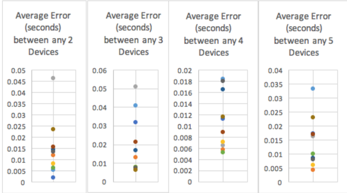
Figure 4-xi: Average error (seconds) for randomly selected devices at beat 27. Each point represents an averaged run in the 32/64 cm group. Each color corresponds to one of the ten runs.
