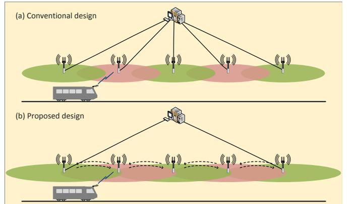
Fig. 2. CBTC trackside network: Conventional vs. proposed design
