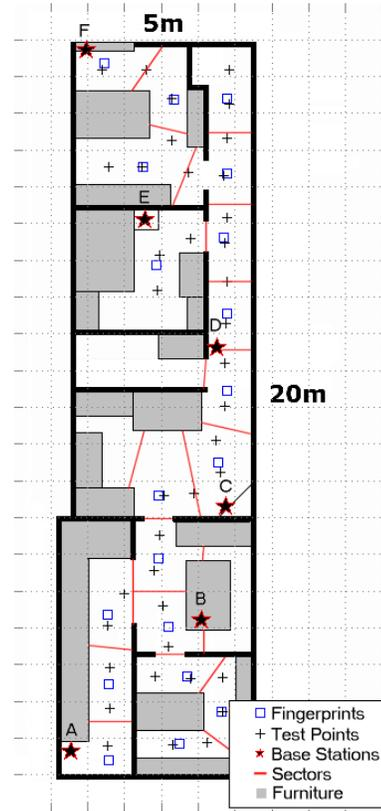
Fig. 1. House test bed, showing fingerprint, test point, and AP locations.
