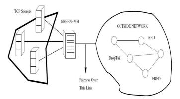
Fig. 1. Green-MH, Located at the boundary of an institution enforcing fairness over the outgoing link
