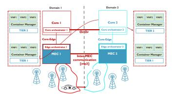
Fig. 1: 5G-CARMEN CCAM architecture: An automated low-latency-aware VNF placement and migration perspective
