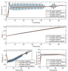
Figure 6: The validation of *adaptive* actor-critic algorithm after training at  $V_{\rm T}(0)=3.6V, T_{\rm cell}(0)=27^{\circ}C$ : (a) *adapted* simplified-states achieves -7.79 cumulative rewards while original simplified-states achieves -81.78 due to state violation; (b) *adapted* full-states achieves -8.19 cumulative rewards while original full-states achieves -82.16 due to state violation.
