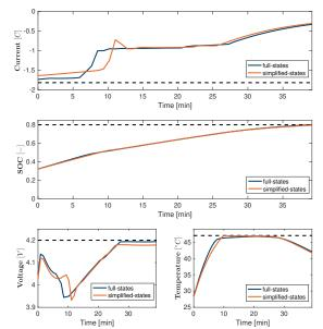
Figure 4: Validation of actor-critic algorithm after training with  $V_{\rm T}(0)=3.6V, T_{\rm cell}(0)=27^{\circ}C$ : (a) simplified-states achieves -5.38 cumulative rewards; (b) full-states achieves -4.69 cumulative rewards.
