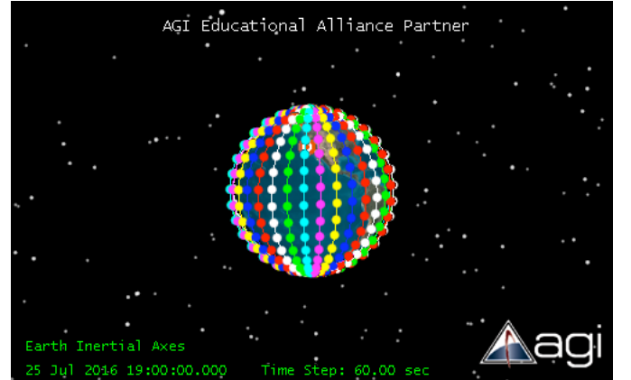
Fig. 9. Polar Constellation of 17 Planes with 33 Satellites per Plane
