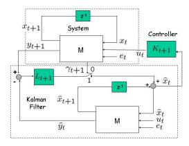
Fig. 1. **Overview of the system.** We study the statistical convergence of the expected state covariance of the discrete time LQG, where the observation, travelling over an unreliable communication channel, can be lost at each time step with probability  $1-\bar{\gamma}$ .
