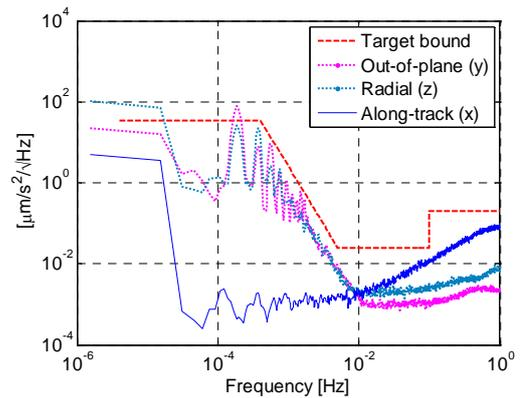
Fig. 9 Spectral densities of the residual CoM accelerations compared to target bound.
