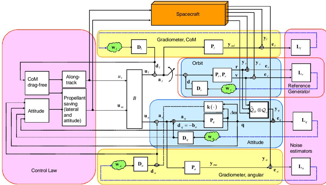
Fig. 8 Block-diagram of the Embedded Model surrounded by Control Law and Noise Estimators.
