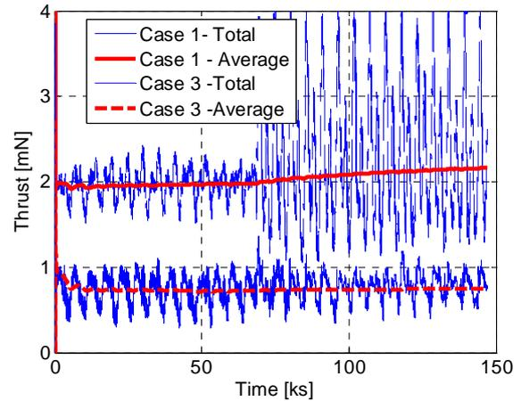
Fig. 14 Cases 1 and 3. Total and average micro-propulsion thrust.
