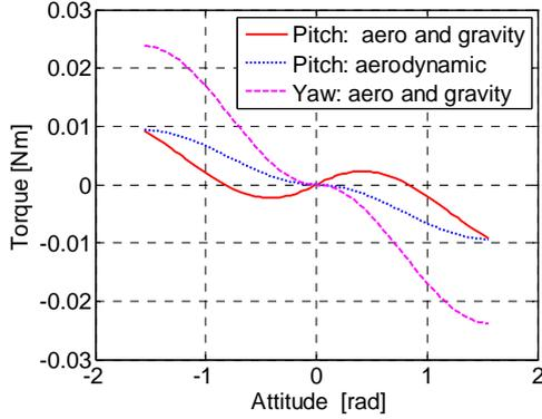
Fig. 7 Aerodynamic and gravity-gradient torques versus attitude.
