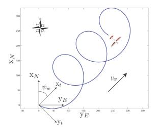
Fig. 2. Trochoidal path and trochoidal frame.
