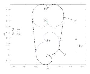
Fig. 3. The dashed line shows candidate extremal paths from initial point and heading to final point and heading. The solid lines are the trochoidal segments at the initial and final states for one full revolution of the airrelative velocity vector.
