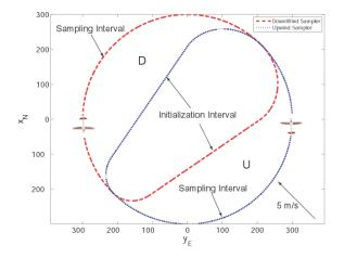
Fig. 4. Two UAVs flying in a time-optimal sampling mission. In the control volume sampling application, UAV1 (UAV2) opens its sample plates only during the upwind (downwind) path segment.
