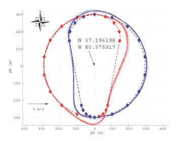
Fig. 5. Experimental results of the path planning algorithm.  $UAV_1$  (blue) sampling only downwind from the source,  $UAV_2$  (red) sampling only upwind from the source. Diamonds indicate GPS waypoints tracked by the onboard autopilot.
