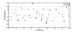
Fig. 6. The effectiveness of the synchronization algorithm as indicated by the phase error (18) between the two UAVs during an aerobiological sampling mission of *P. infestans*. The average phase error was  $5^{\circ}$ .
