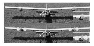
Fig. 1. A UAV with sample collection plates closed (top) and open (bottom) [6]. In the control volume sampling application, the plates are opened only during the sampling interval.
